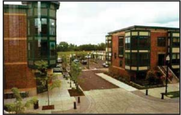
Parking areas can be located behind buildings to keep the street oriented to pedestrians. Orenco station, Hillsboro, OR
